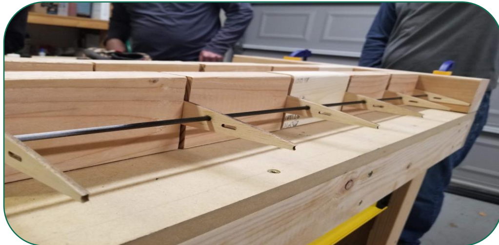
Wing jig used to epoxy ribs
